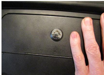
3. Holding the door in place with one hand, insert one of the self-tapping screws into a hole. Pay attention to center the screw in the hole with a screw
