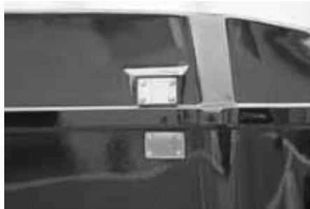
2. Using a 5/32" drill bit, steady the plate with one hand and carefully drill 1 hole. Install one machine screw and nut and tighten slightly to stabilize the plate's location. Drill a 2<sup>nd</sup> hole and install a 2<sup>nd</sup> screw and nut. Complete drilling the remaining two holes. Remove plate, screws and nuts.
