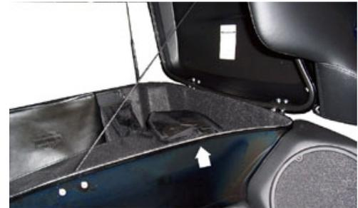
2. Using a 5/32" drill bit, steady the plate with one hand and carefully drill 1 hole. Install one 1/2" machine screw and nut and tighten slightly to stabilize the plate's location. Drill a 2<sup>nd</sup> hole and install a 2<sup>nd</sup> screw and nut. Complete drilling the remaining two holes. Remove plate, screws and nuts.
