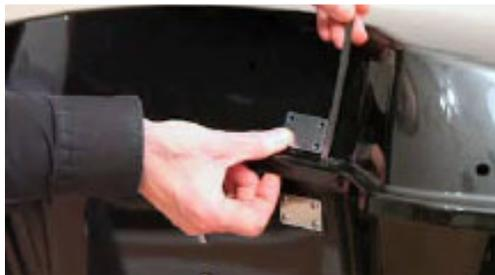
6. Drill 4 holes using the procedure in step 4.
